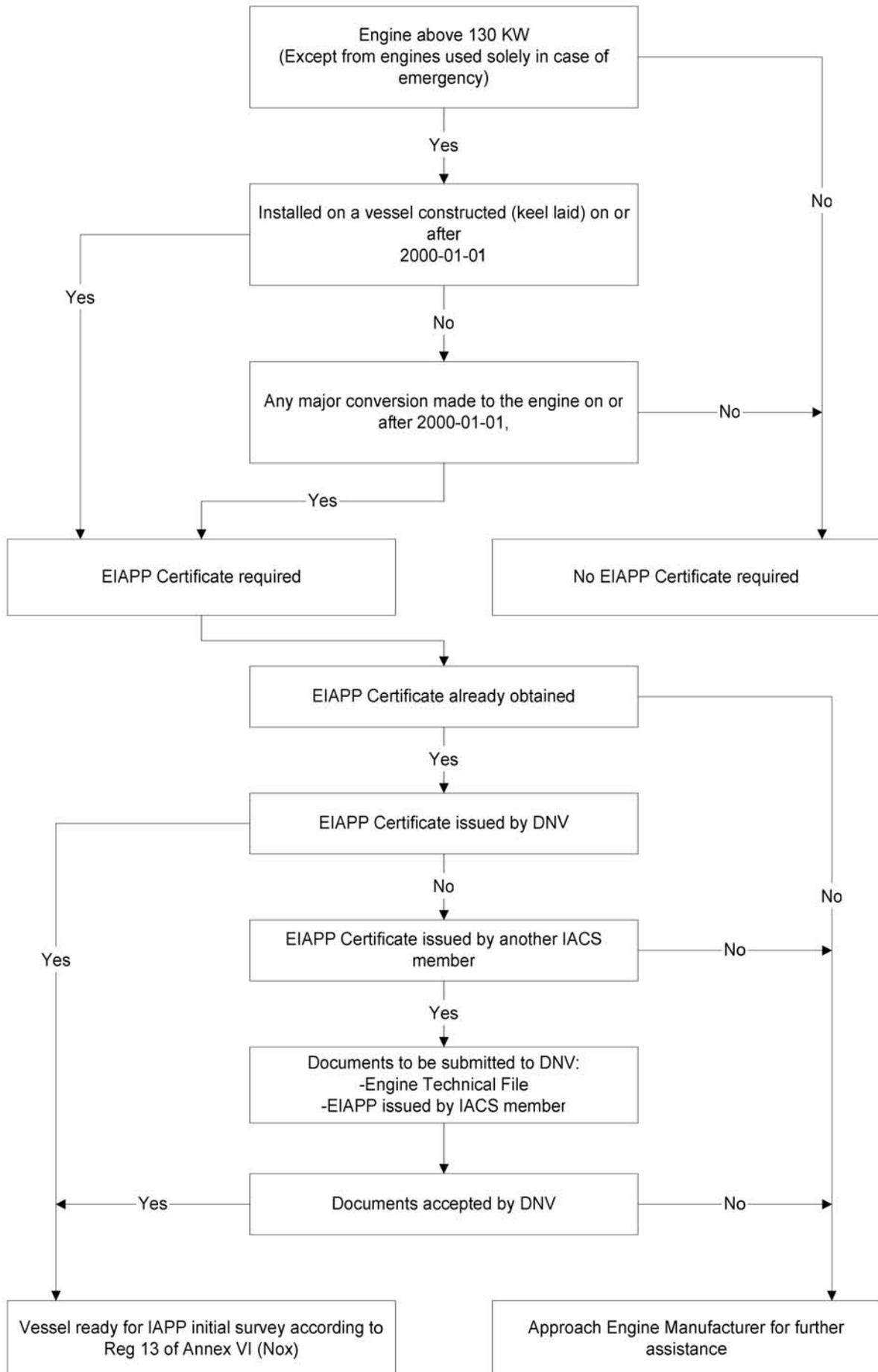
The flow chart above is meant as a general guidance indicating the necessary steps for you to consider regarding the NOx requirements of Annex VI. Please note that the flow chart is only concerning the NOx requirements to the diesel engines, and this is also what the EIAPP certificate is covering.
